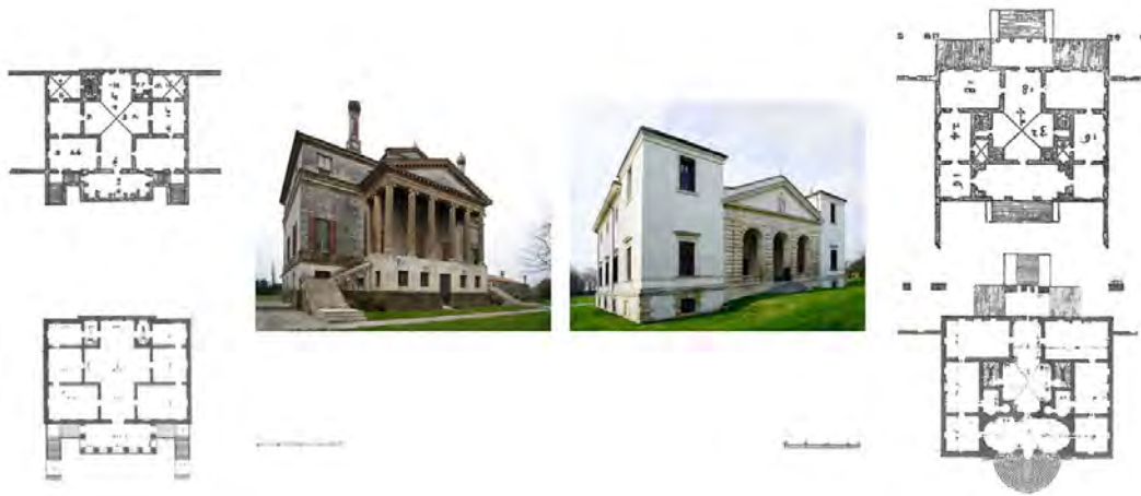
Fig. 2 – Villa Foscari and Villa Pisani in photographs and as depicted by Palladio (top) and Scamozzi (bottom). The plans shown in the same scale illustrate Villa Foscari has a smaller footprint than Villa Pisani but is taller. Palladio's version as presented in his Four Books of Architecture shows his ideal and is different from the measured condition described in Scamozzi's drawing, which is also different from the present day recording.
