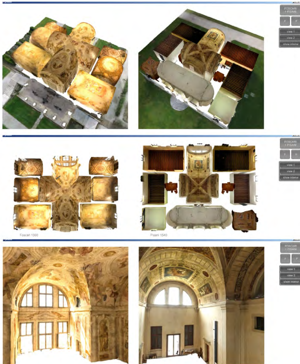
Fig. 12 – Comparison of ceiling structure and texture of the Villa Foscari (left) and Villa Pisani (right). Images on the top show the ceiling textures mapped on the reversed side and seen from above. (Copyright: Nagakura, Tsai and Pinochet)
