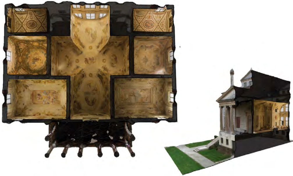
Fig. 1 – Photogrammetric model of Villa Foscari's fresco vaults viewed from below and in section. (Copyright: Nagakura, Tsai and Pinochet)
