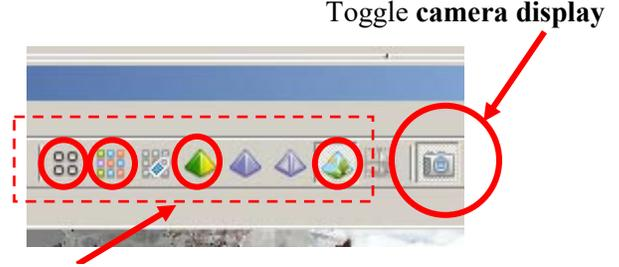
From left to right: **Tie Point Model**, **Dense Cloud Model**, **Shaded Model**, and **Textured Model**
