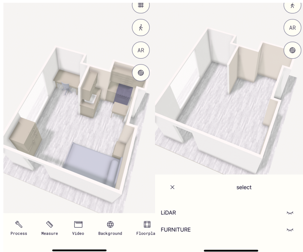
Figure 3.7. (a) 3D scan result of PolyCam (b) resulting layout after hiding furniture. From (Polycam - LiDAR & 3D Scanner for iPhone & Android, 2024)
